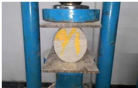
Fig 4: Split Tensile Strength Test
