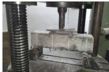
Fig 5: Flexural Tensile Strength Test
