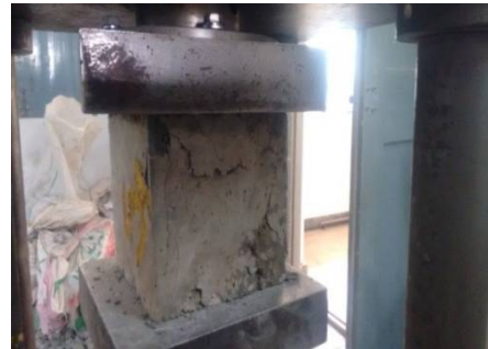
Fig 3: Compressive Strength Test
