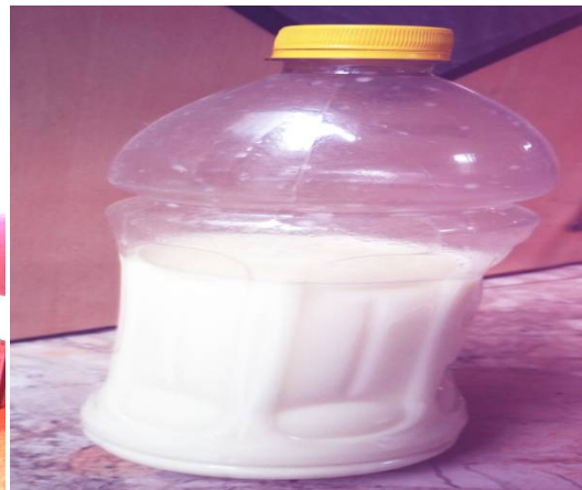
Photo No.2 Karanja oil in water based cutting fluid
