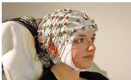
Figure 1: A test subject participating in a BCI experiment. Note the EEG electrodes attached to the cap.
