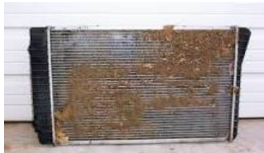
Fig (II) Clogged Radiator
