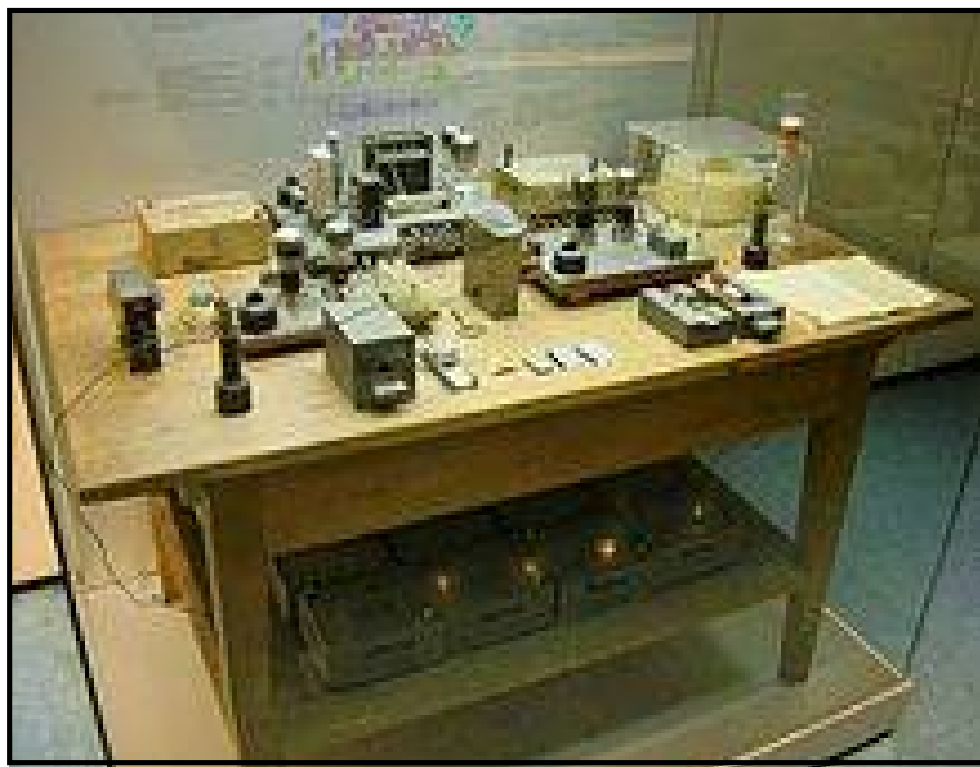
Fig.6 The experimental set-up of Hahn and Strassman for nuclear fission in 1938
