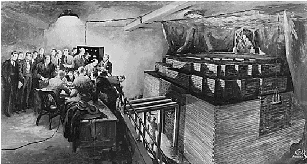
Fig.26. Team of scientists working with the Fermi's Pile (Cadmium rods are being removed from the core)
