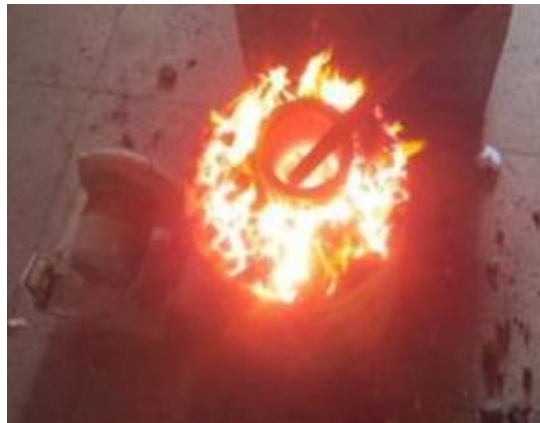
Fig 2 Manual Stirring of Composite Slurry in Crucible of Coal Fired Furnace
