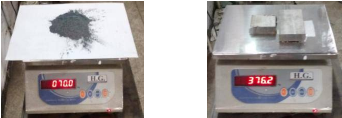
Fig 1 Weighing of SiC and Commercial Aluminium on Weighing Machine
