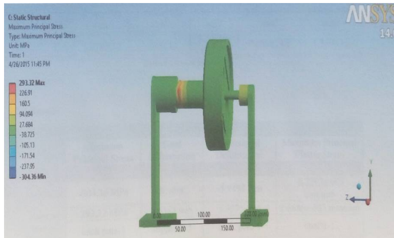
Fig. 8 Maximum Principle stress of Rigid body type clutch
