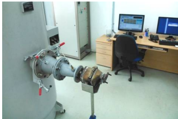
Fig. 10 Converter - Pressure drop measurement test setup
