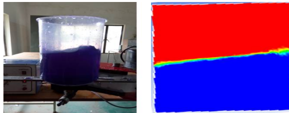
Fig. 18: Comparison of Free Surface Profiles at t=2 \text{ sec} ( \omega = 1.74 \text{ rad/sec} )
