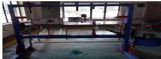
Fig.16: Dunkerley'sVibration Measuring Apparatus
