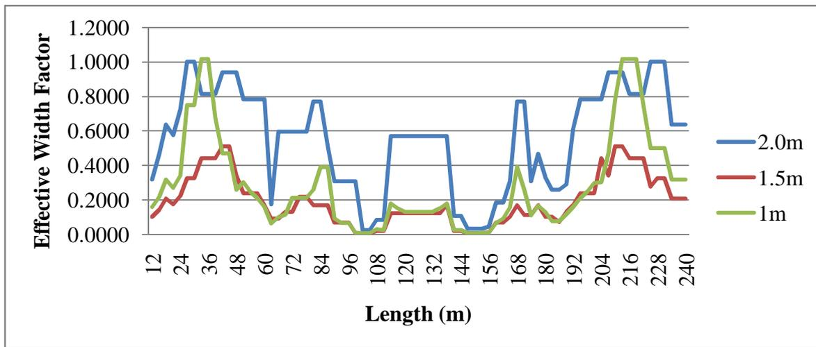
Figure No. 4 Comparison of effective width factor for different sizes of cross girder
