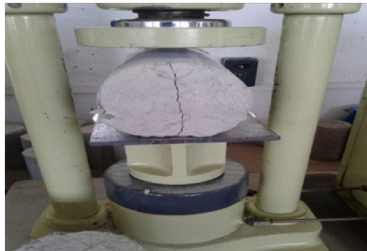
Fig 5.2 Split tensile strength test
