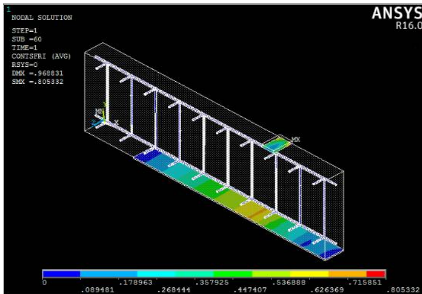
Fig 3. Contact friction stress for 5 mm thick CFRP
