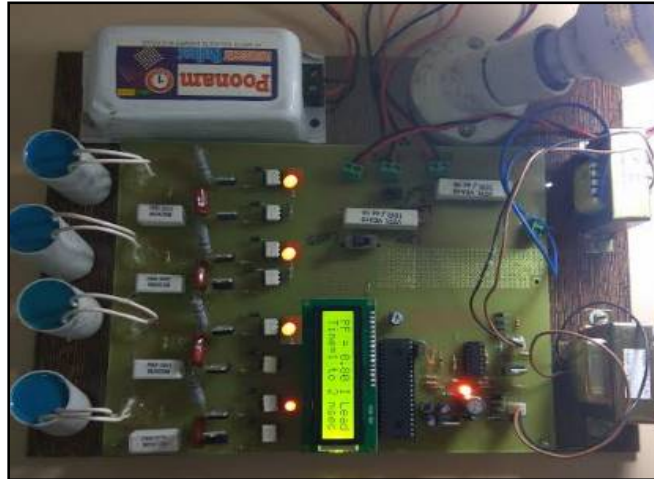
Fig.6 Output in LEAD position with improved PF
