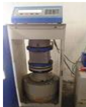
Fig 4.3. Compression testing machine
