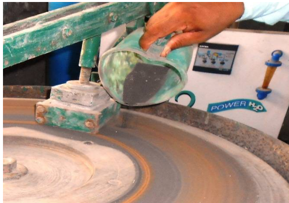
Fig no 5: Abrasive Powder on the rotating disc
