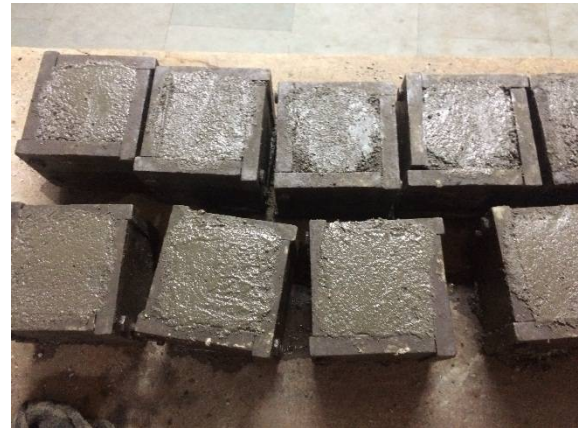
Fig no 6: Mortar samples in the mould
