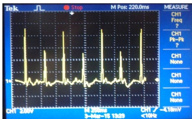
Figure 4: Pulsating Output Voltage of Piezo under pressure Charging circuitry
