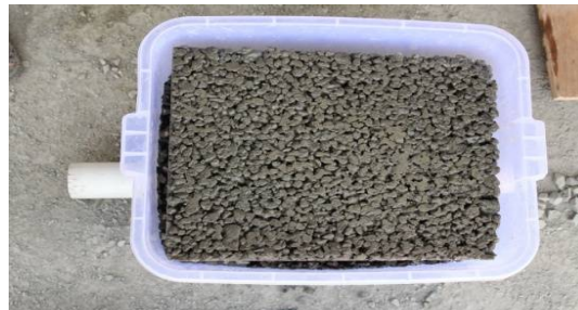
Fig -5: Porous concrete system
