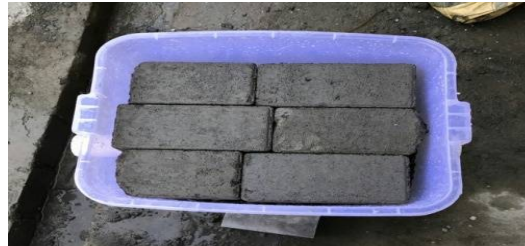
Fig -3: Permeable paving block system
