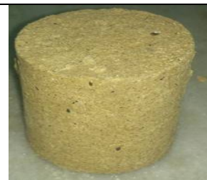
Figure 10: Briquette of Saw dust and Corn Starch
