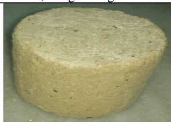
Figure 9 :Briquette of Saw dust & Wheat flour
