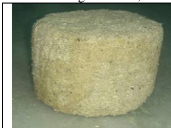
Figure 8 : BRIQUETTE OF SAW DUST
