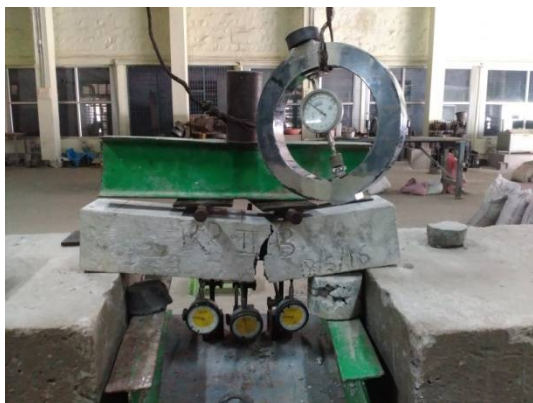
Flexure test after 28days curing
