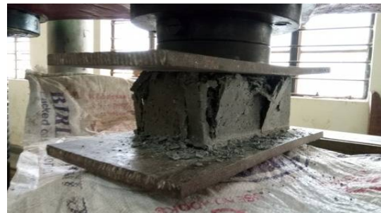
(e) The Brick Specimen after Failure.
