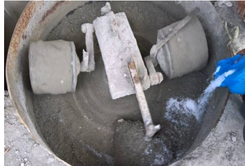
b) The Shredded polyethylene being added to the mixture
