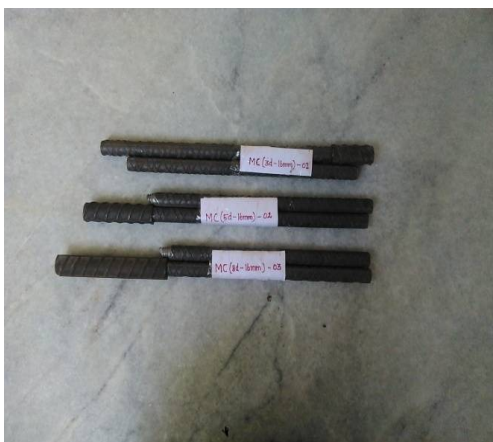
Fig 4: Coupled bars (12mm and 16mm)
