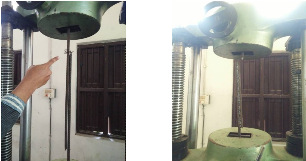
Fig 3: Testing of welded and development bars
