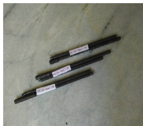
Fig 4: Coupled bars (12mm and 16mm)
