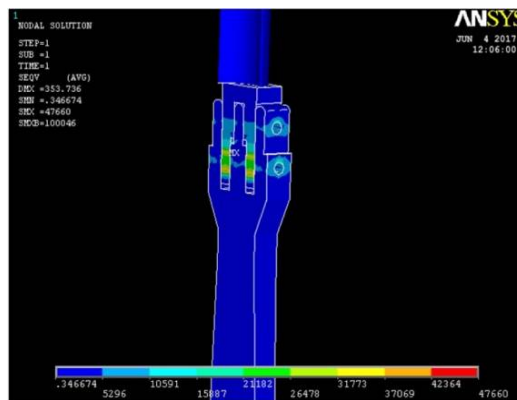
Fig.9 Von mises stress for 3600rpm
