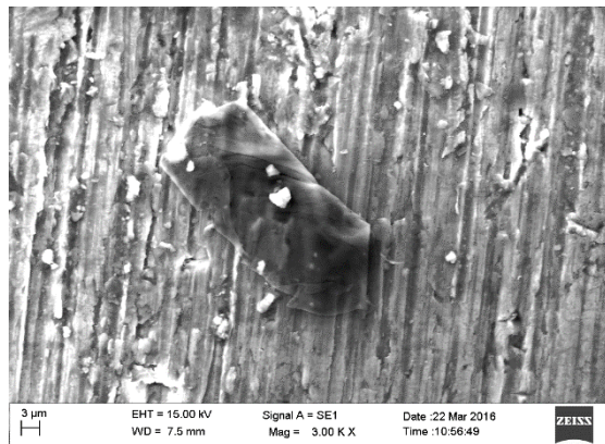
Fig. 1 SEM image of 4 % B_4C particulate reinforced AA6061 composite.
