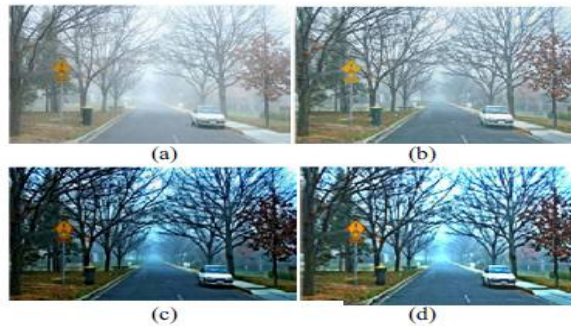
Figure 2: Fog removal from video (a), (b) & (c) input videos and (d) is output video
