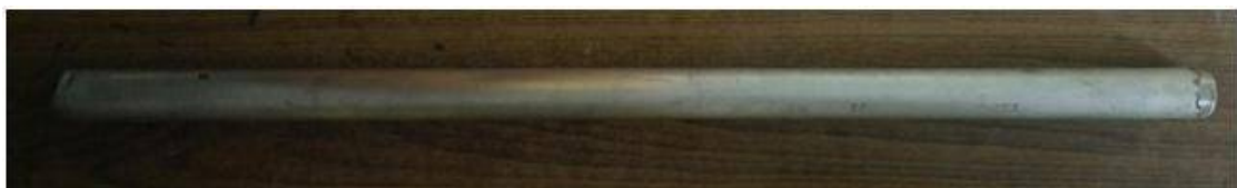
Fig. 2 Aluminum Tube Partially Collapsed
