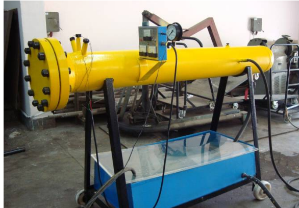
Fig. 1. External Pressure Testing Equipment
