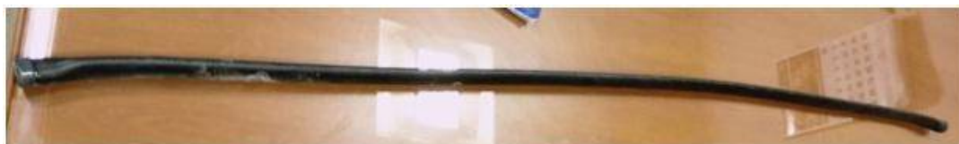
Fig. 6 Deformed Composite Pipe II
