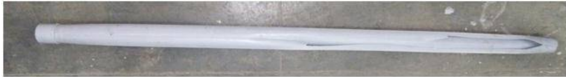
Fig. 3 Broken PVC Pipe
