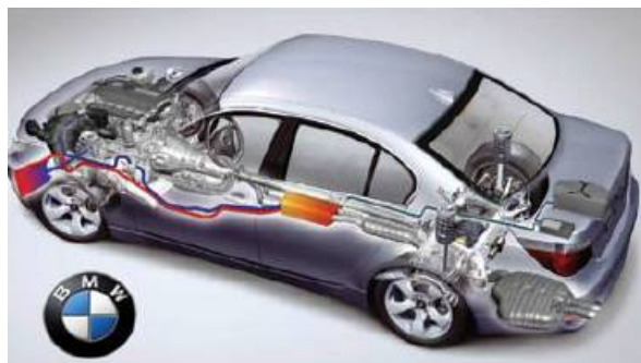
Fig. 4. Conceptual design of thermoelectric generator producing electricity from waste heat in the engine exhaust. [26]
