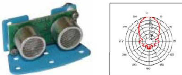
Figure 2 : Sensor and its emission pattern
