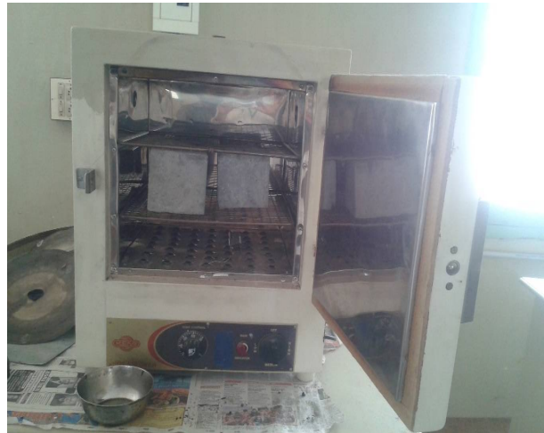
Fig .1 Oven Heating @ 110°C for 1 hour
