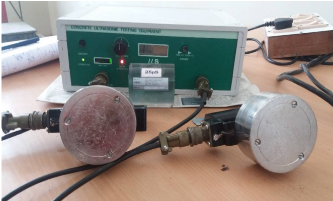
Fig .2 USPV Testing machine
