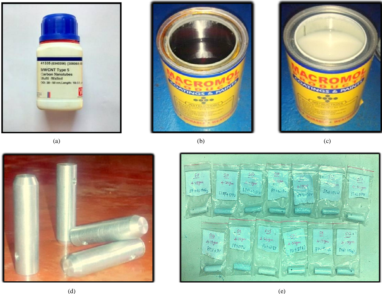
Fig. 1 Sample preparation requirements (a) Multi-Walled Carbon Nanotubes OD 30-50 nm (b) Epoxy Polyamide-Primer (c) Polyurethane-Top Coat (d) Aluminium alloy compatible to coat and test wear (e) Various coated samples of differed compositions
