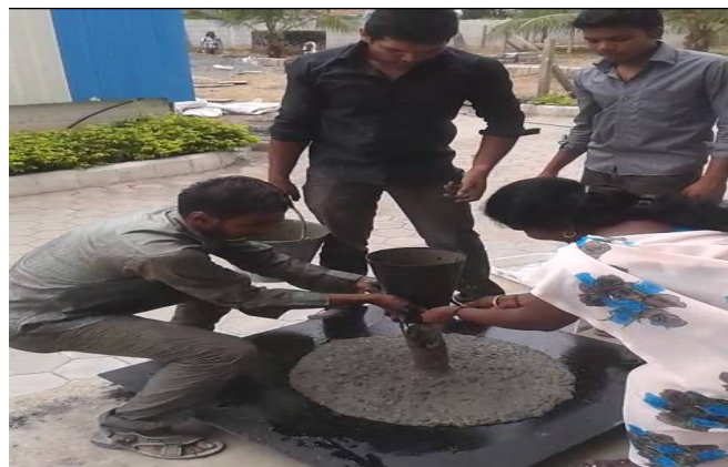
Fig. 2: Slump flow test
