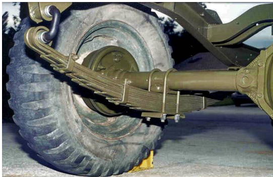
Fig 2.a Arrangement of leaf spring in automobile
