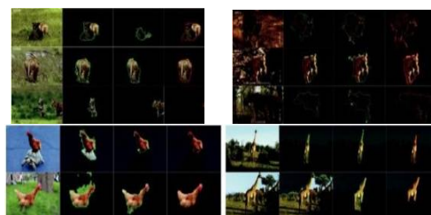
Fig. 3. Segmentation examples of the proposed method and two comparison methods [7], [17]. In each sheet, the first column presents the original video frames; from the second to the fourth columns, the segmentations of [7] and [17] and our method are displayed, respectively.
