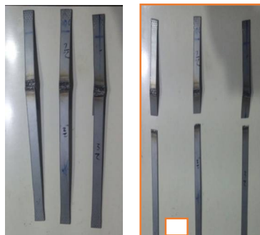
Fig. 3. Tensile test sample images (a) before the tensile test (b) after the tensile test
