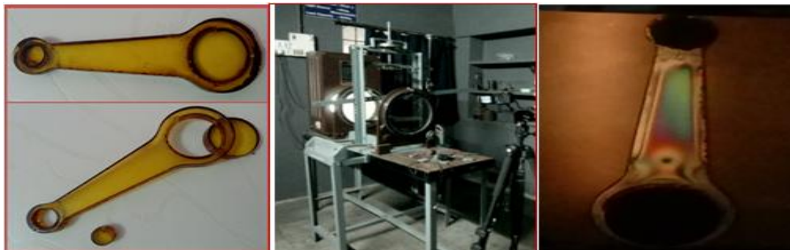
Figure: 04 Connecting rod Specimen, Experimental setup
