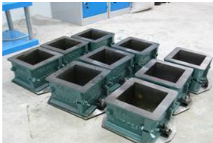
Fig (a) Moulds for compressive strength determination
