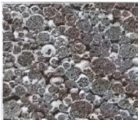
Figure 2: Lightweight Aggregate Concrete
