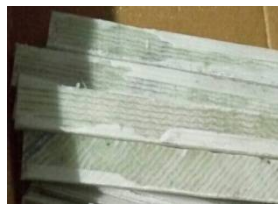
Fig. 3a – Tray (on left), 3b - Prepared Glass fiber laminates (on right) Fig. 4 Prepared specimens of Glass Epoxy Laminate after cutting
