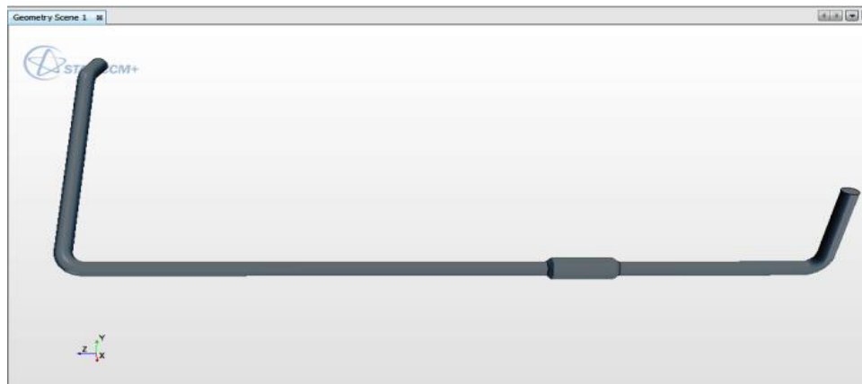
Figure 3: Model of with inlet, outlet and substrate in STAR-CCM + .
