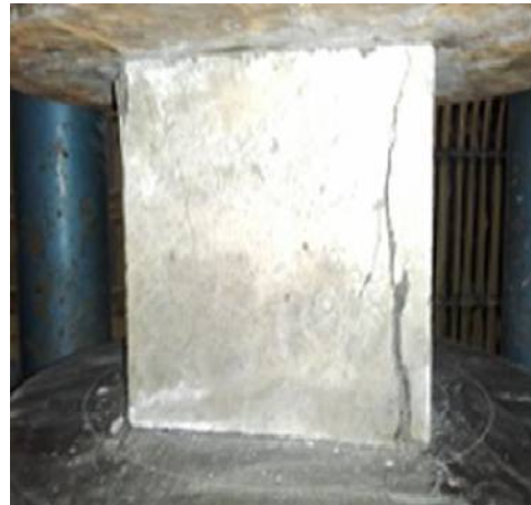
CONCRETE CUBE SPECIMENS TESTING FOR COMPRESSIVE STRENGTH
