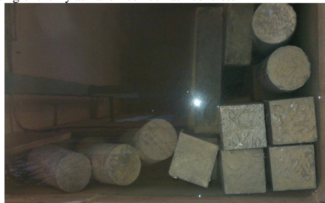
NWC USED FOR CURING OF CONCRETE SPECIMENS
