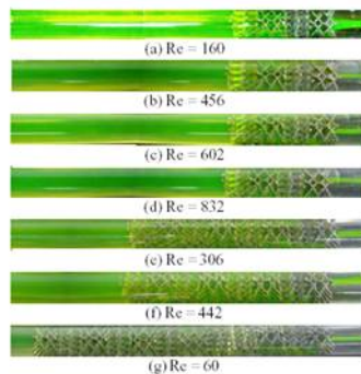
Figure 3: Flow visualization Results, (a,b,c,d), 8 Mixers (e&f) 12mixers (g) flow right to left.
