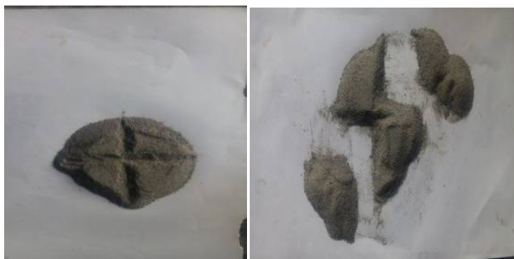
Fig.2 Cone and Quartering Method for SEM Sample Preparation
