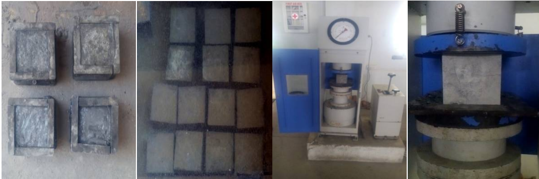
Fig.1 Casting, Curing and Testing of Concrete
