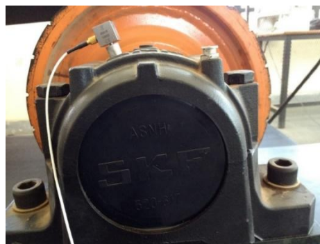
Fig.1 Accelerometer mounted on plummer block casing
