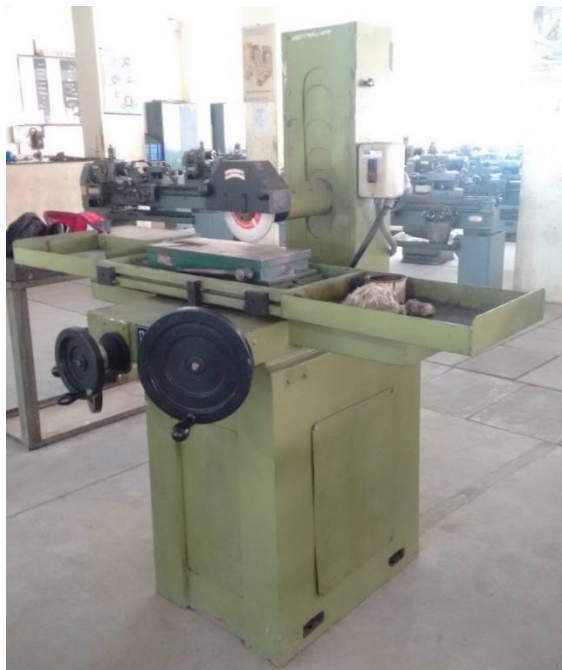
Fig 1. The surface grinding process
