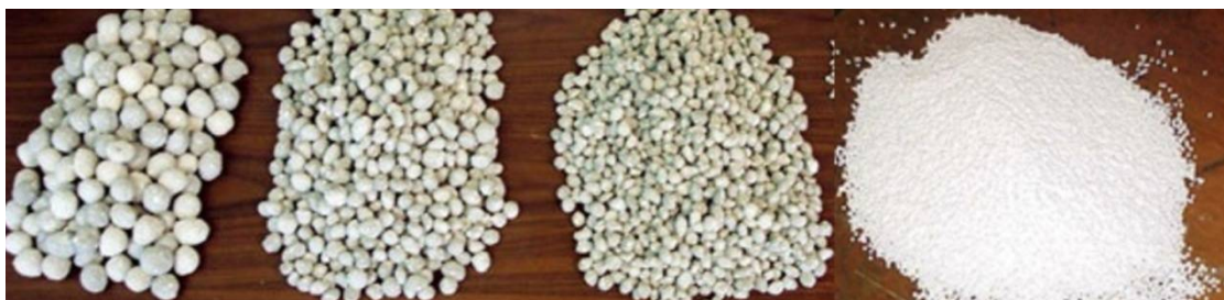
Figure 1: 20 mm, 12.5 mm, 10 mm MEPS coarse aggregate and MEPS fine aggregates
