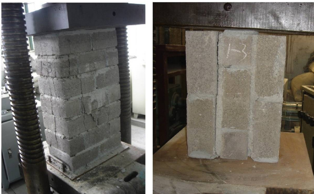
Figure 4: Cracking mode of masonry prism in compression and Failure mode of shear test
