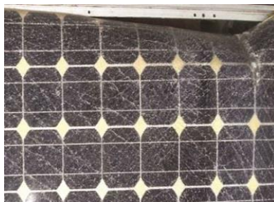
Figure 3(b): Deframing of solar module
