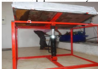
Fig. 2- Photographic view of lifting of trailer in one direction
