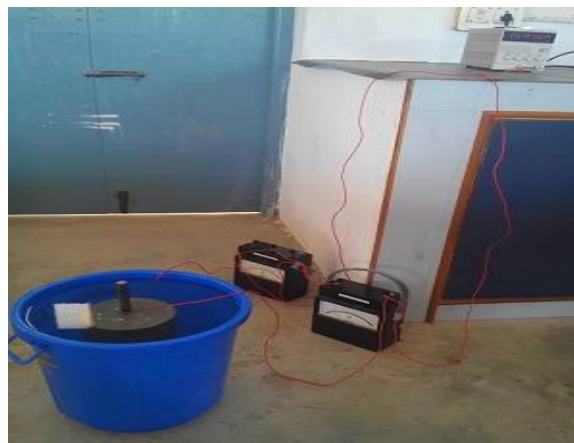
Figure 6.5 Accelerated corrosion Test
