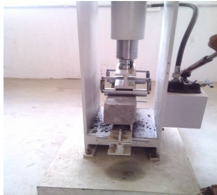
Figure 5.4 Flexural strength test
