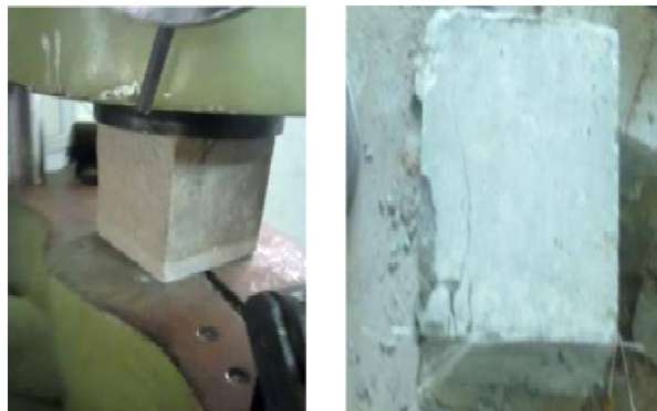
Figure 5.2 Compressive strength test
