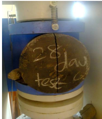
Figure 5.3 Split tensile strength test
