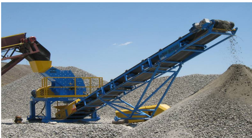
Figure 4: Conveyors for transporting crushed rock waste material (Source: Living-lifestyle, 2014)
