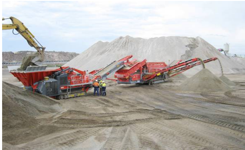
Figure 5: VSI Crusher used for glass recycling into sand product (Source: Living-lifestyle, 2014)
