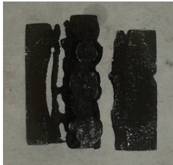
Fig. 7: State of welded joint exposed to 1M H 2 SO 4 .
