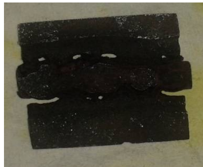
Fig .6: State of welded joint exposed to 0.5 M H 2 SO 4 .
