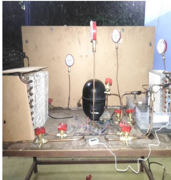
Fig 4.9 Photo copy of refrigeration system with micro channel condenser, but this proposed vapour compressor refrigeration system working under the round tube and also micro channel condenser in swapping with capillary and Thermostatic expansion devices.
